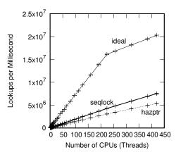
Figure 9.5: Pre-BSD Routing Table Protected by Sequence Locking
