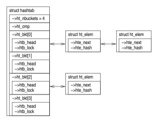
Figure 10.1: Hash-Table Data-Structure Diagram
