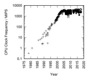
Figure 6.11: MIPS/Clock-Frequency Trend for Intel CPUs
