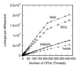
Figure 9.21: Pre-BSD Routing Table Protected by RCU
