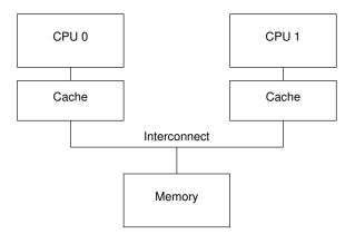
Figure C.1: Modern Computer System Cache Structure
