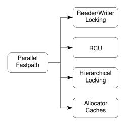
Figure 6.18: Parallel-Fastpath Design Patterns
