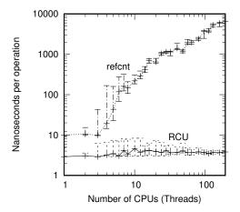
Figure 9.31: Performance of Preemptible RCU vs. Reference Counting
