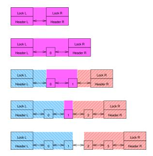
Figure 6.5: Double-Ended Queue With Left- and Right-Hand Locks
