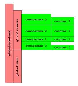
Figure 5.5: Simple Limit Counter Variable Relationships
