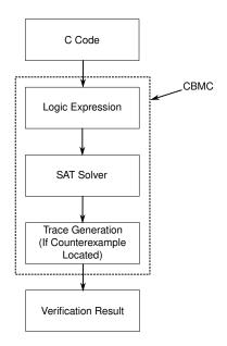
Figure 12.2: CBMC Processing Flow
