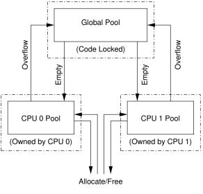
Figure 6.19: Allocator Cache Schematic
