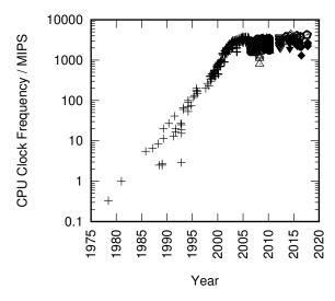
Figure 2.1: MIPS/Clock-Frequency Trend for Intel CPUs
