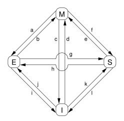
Figure C.3: MESI Cache-Coherency State Diagram
