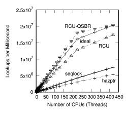
Figure 9.22: Pre-BSD Routing Table Protected by RCU QSBR
