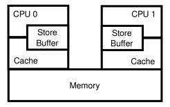
Figure 15.1: System Architecture With Store Buffers
