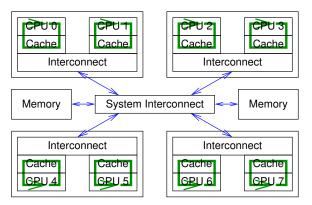
Figure 5.4: Data Flow For Per-Thread Increment
