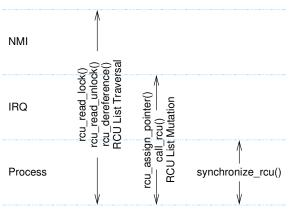
Figure 9.20: RCU API Usage Constraints
