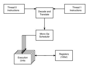
Figure 3.4: Rough View of Modern Micro-Architecture
