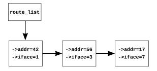
Figure 9.1: Pre-BSD Packet Routing List
