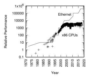
Figure 6.12: Ethernet Bandwidth vs. Intel x86 CPU Performance
