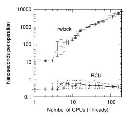
Figure 9.25: Performance Advantage of RCU Over Reader-Writer Locking
