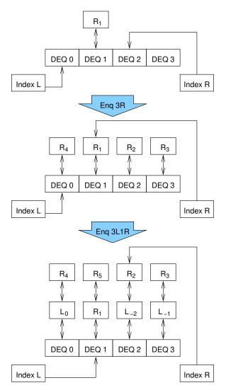
Figure 6.8: Hashed Double-Ended Queue After Insertions
