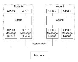
Figure C.8: Example Ordering-Hostile Architecture
