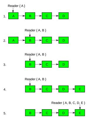
Figure 9.15: Multiple RCU Data-Structure Versions
