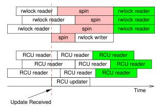
Figure 9.28: Response Time of RCU vs. Reader-Writer Locking
