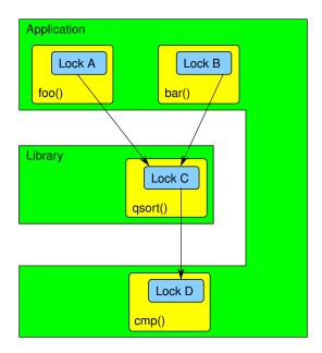
Figure 7.7: Layered Locking Hierarchy for qsort()
