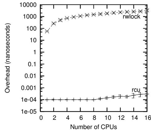
Figure 9.23: Performance Advantage of RCU Over Reader-Writer Locking
