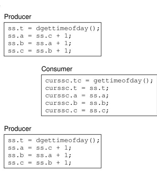
**Figure A.1:** Effect of Locking on Snapshot Collection
