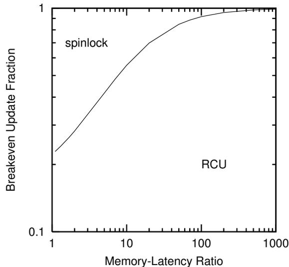
**Figure 17.6:** Breakevens vs.  $r$ ,  $\lambda$  Large, Four CPUs
