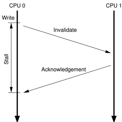
**Figure C.4:** Writes See Unnecessary Stalls
