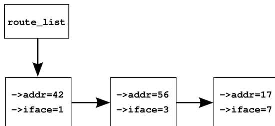
**Figure 9.1:** Pre-BSD Packet Routing List
